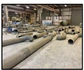
The last shipment for the Lancer Sports Stadium in Windsor, Ontario was installed. This recreation center featured UnderDuct in both single wall and double wall R-6 construction. This underground pool duct system contained round UnderDuct sizes up to 48" diameter and a total of 58 register boots.
